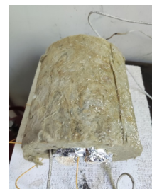
Fig. 2. Device for researching the thermal conductivity of wood polymer material: 1 – wood polymer material; 2 – cylindrical heater; 3 – thermal insulation; 4 – thermocouples; 5 – temperature recording device
