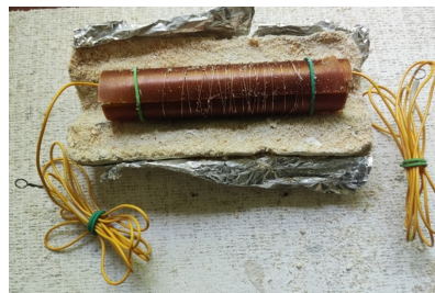
Fig. 2. Device for researching the thermal conductivity of wood polymer material: 1 – wood polymer material; 2 – cylindrical heater; 3 – thermal insulation; 4 – thermocouples; 5 – temperature recording device
