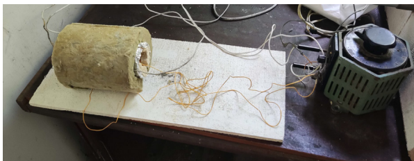
Fig. 5. The process of determining the thermal conductivity of a wood polymer sample under the influence of a heater
