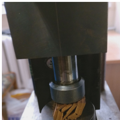
Fig. 12. Determination of the compressive strength of wood
