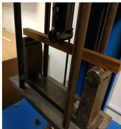
Fig. 10. Determination of static bending strength of wood
