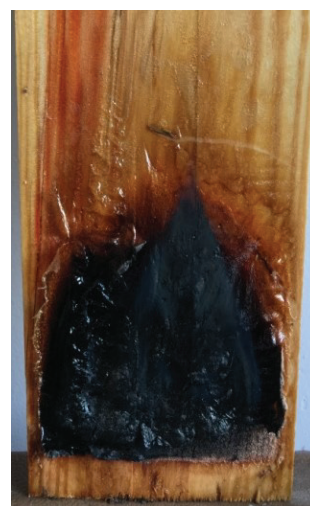
Fig. 6. Swelling of the fire-retardant varnish during thermal action
